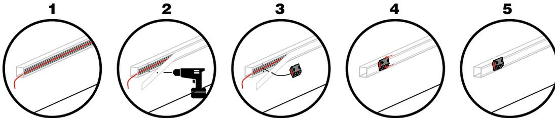
TS-SR-T24 rail installation example in trunking
