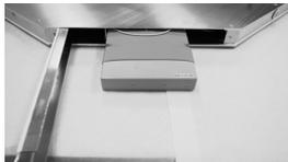
5. Unplug battery to PCB leads from top of battery and connect to new battery pack.
